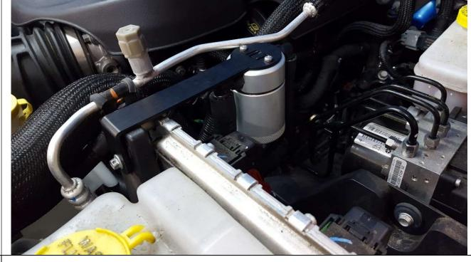
REMOVE ENGINE COVER BY PULLING STRAIGHT UP AND PULL FORWARD. Route hoses under intake tube and throttle body up into the intake manifold area. Unplug hard PCV line from angled rubber connection. Plug J&L line with male fitting into the rubber angled connection and the rubber female to the factory hard line shown here:
